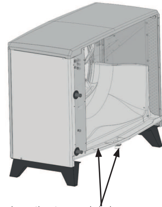
Condensation tray and drain
