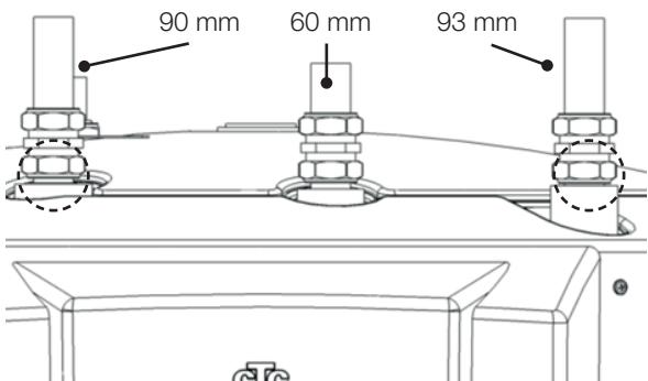
3. Unscrew the 90-degree- and T-coupling, together with the copper pipes. The copper pipes do not have to be disassembled from the couplings. Leave the lower nuts as they fit the couplings in the next assembly step.
