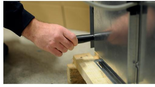
2. Attach the two carrying handles to the bottom of the cooling module.
