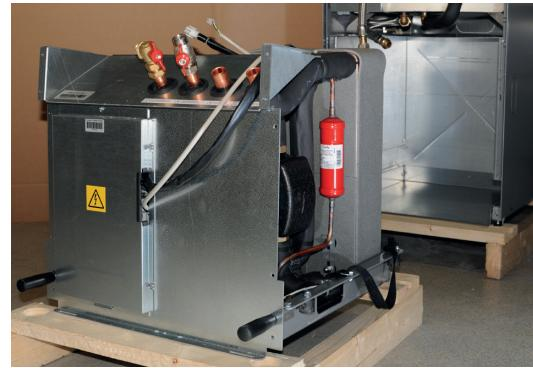
6. Lift the cooling module into the product using the carrying handles and shoulder straps. Remove the carrying handles and reconnect the power cable, hoses and screws.
